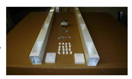
On the gate post put pvc glue into the gate pocket and slide each rail into pocket. It will be a very tight fit and you must not take to much time or the glue will dry.
