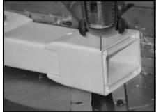
(2c) Now it's time to cut your rails. Slide bracket covers off of your rails and cut on the inside of your marked lines. This will allow for the 1/8 width of the aluminum brackets. Cut your bottom rail. Repeat on your top rail with the aluminum reinforcement inside top rail with picket stabilization beads facing picket holes.
